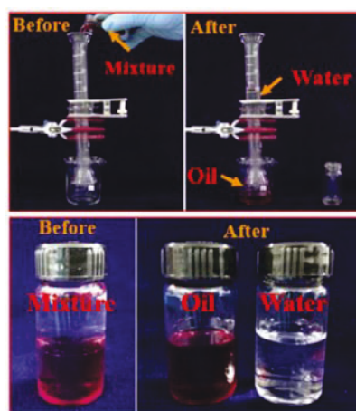
Figure 6. The separation process for oil/water mixtures
