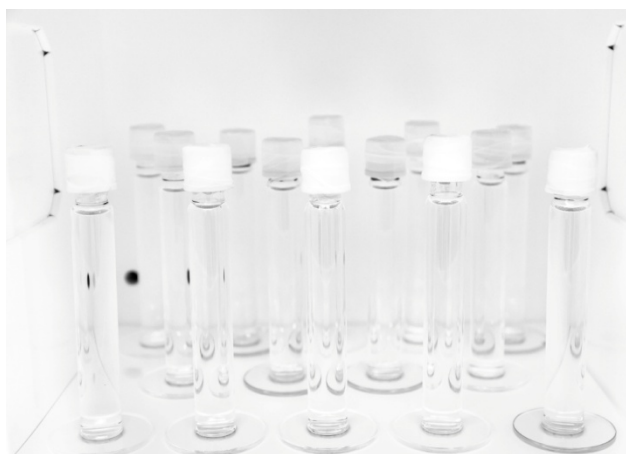
Sample vials in the light chamber (top and bottom left) and with a ruler for scale (right). Caps are wrapped with PTFE tape to increase reflectance and thereby minimize heating of the vials during UV irradiation. A typical TDP run has 18 vials in the light chamber and a typical TDN run has 24 vials.
