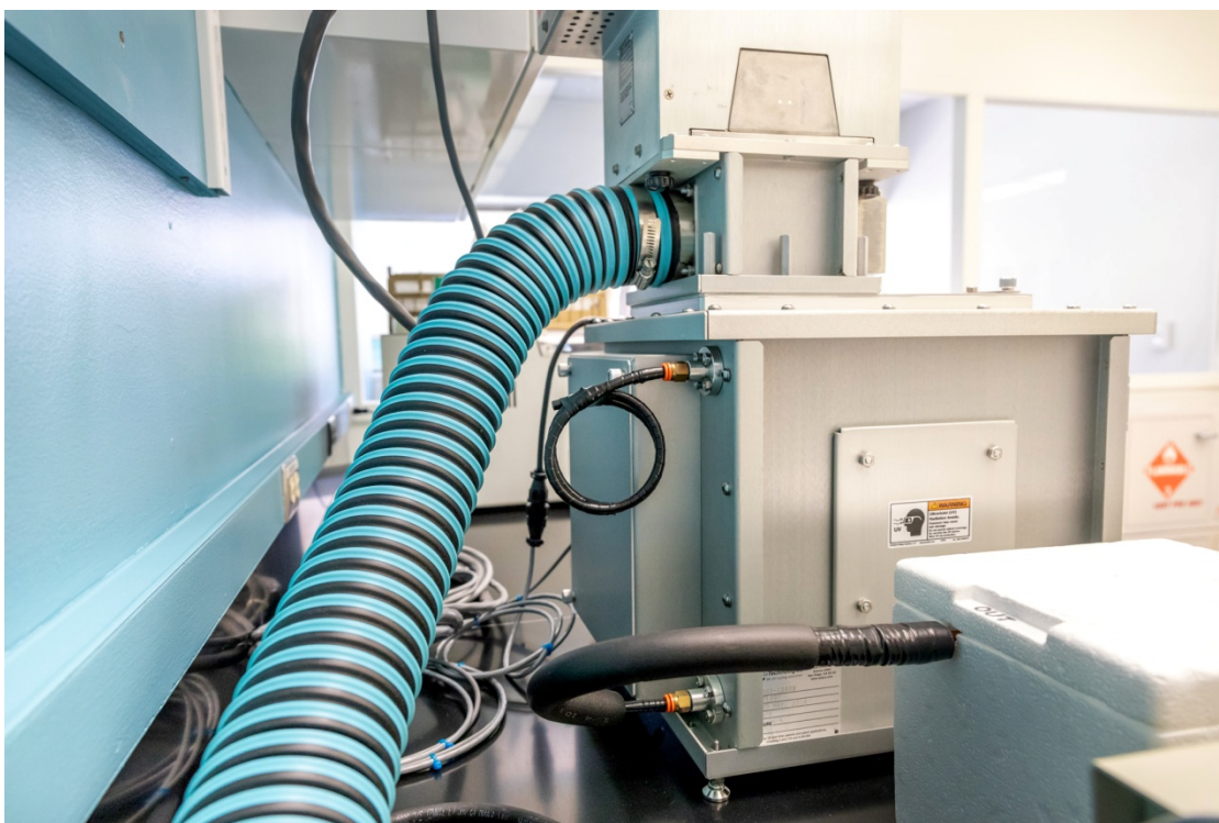
Rear of system, showing sample cooling air going into the bottom back port of the light chamber and 3 in. ducting extending from the light assembly and heading to the exhaust/cooling fan in the hood.
