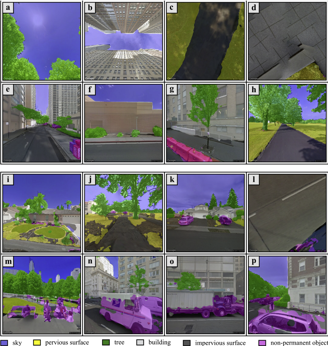
Fig. 6. Sample image segmentation results illustrating segmentations with an accuracy > 95% (a-h) and an accuracy < 95% (i-p).
