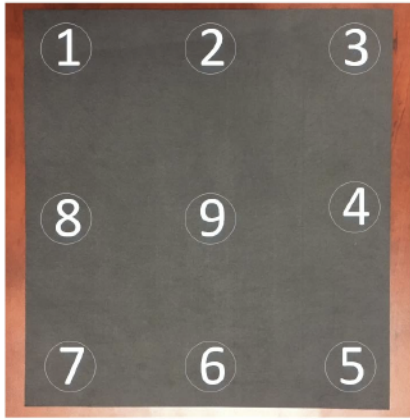
Fig. 4. The consistency test of the piezo-resistive material. The numbers from 1 to 9 indicate the locations of the testing points on the material.
