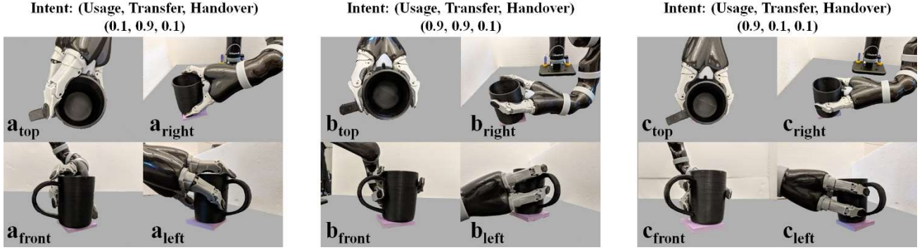
Figure 5: There are three separate grasp poses a) represents the pose which satisfies the transfer task and not the other two tasks as seen by the intent provided on the top. This grasp dominates the top of the cup to leave room to place and it is unsuitable for usage. b) is the pose which our model generated which carries the subtleties to satisfy both usage and transfer while not satisfying handover. The robot hand dominates the handle by having a majority of fingers around it, while leaving sufficient room to drink from the top. The palm is higher on the cup. c) is the pose for which satisfies the usage task. The fingers dominate the handle space by having a majority of fingers near the handle, sufficient room on the top for drinking.
