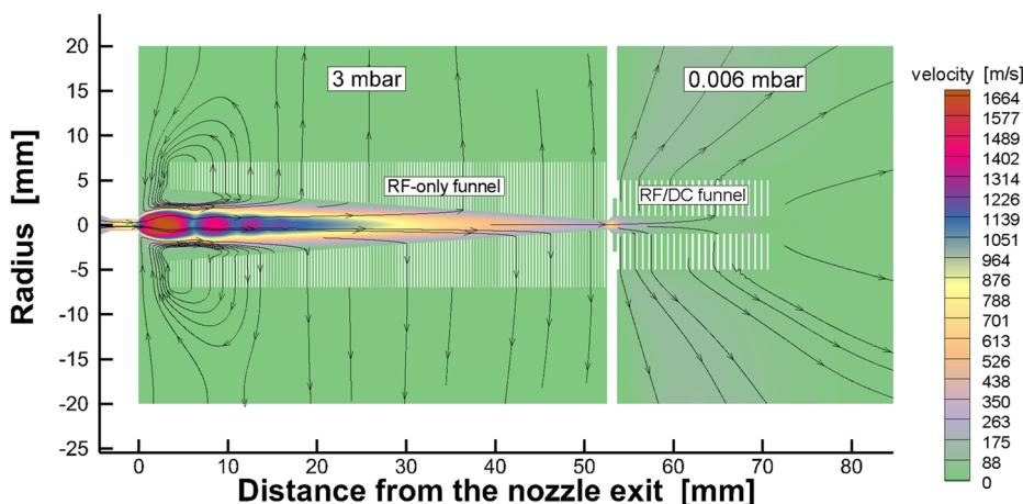
**Fig. 2** Gas dynamic simulation of the double-RF-funnel extraction system for the gas velocity flow field
