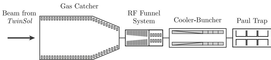
**Fig. 1** Schematic diagram of the design of St. Benedict, showcasing the four major elements: the gas catcher, RF funnel extraction system, cooler-buncher, and Paul trap
