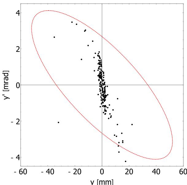
**Fig. 4** Comparison of emittance of ion beam on injection into the Cooler-Buncher (black points;  $\epsilon_{\text{RMS}} = 21\pi$  mm mrad) with the acceptance of the Cooler-Buncher (red, dashed line;  $\epsilon = 139\pi$  mm mrad)
