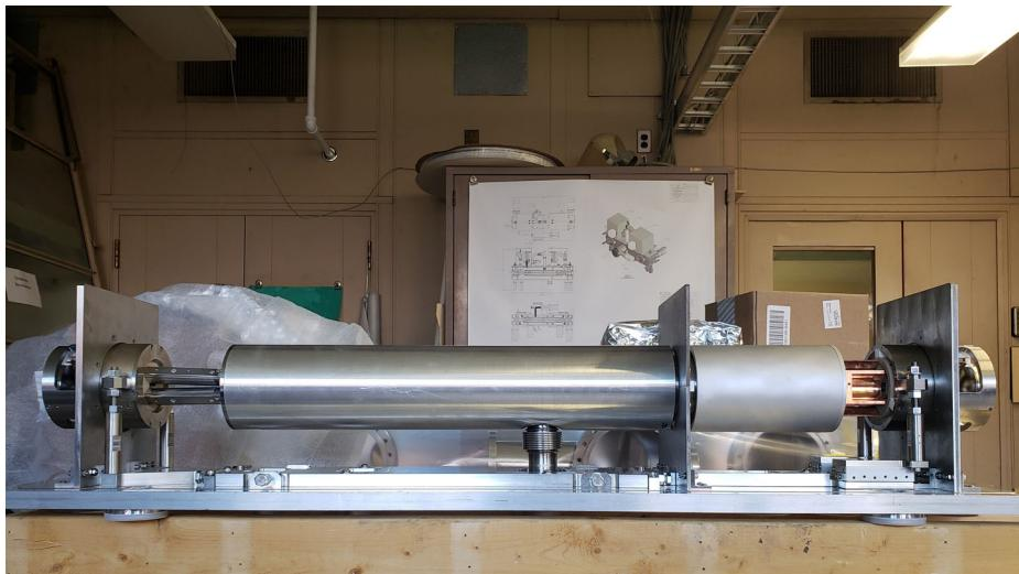
**Fig. 5** Photograph of the assembled internal structure of the cooler-buncher before the wiring of the electrodes, including enclosed cooling section, differential pumping barriers for the different pressure regions, and assembly of the electrode structure including flared injection RFQ electrodes and diagonally-split cooling region electrodes. Beam travels from left to right
