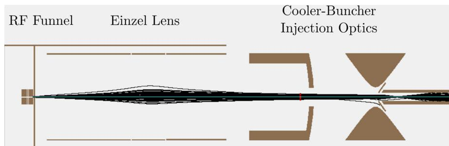
**Fig. 3** SIMION simulation of ion optical transport from the double-RF-funnel system to the Cooler-Buncher using an Einzel lens
