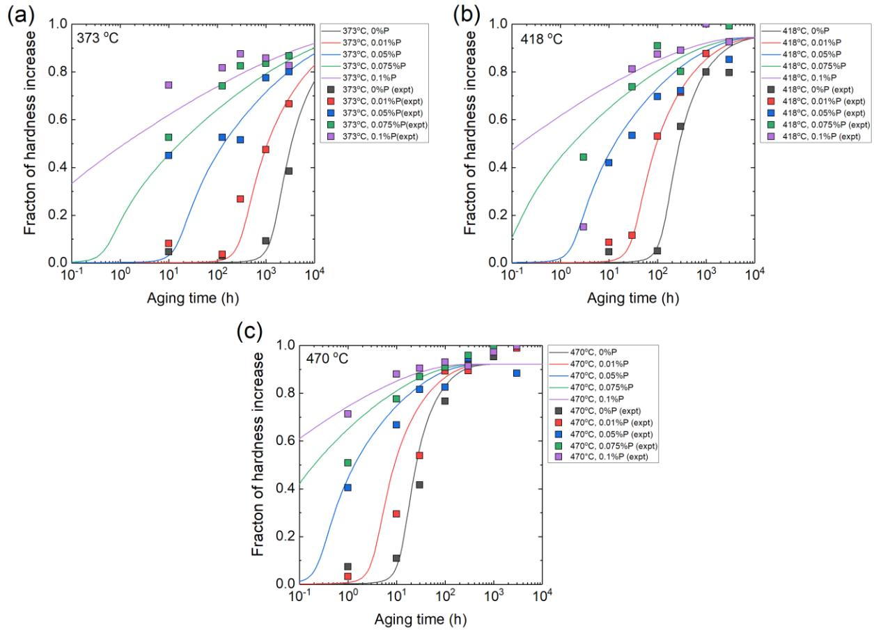
Figure 7. Plots showing the fraction of hardness increase as a function of isothermal aging time for Ni-33%Cr alloys with 0, 0.01, 0.05, 0.075, and 0.1 at.% phosphorus at (a) 373 °C, (b) 418 °C, and (c) 470 °C. The symbols show the data from experiment and the line plots show the result of Dienes ordering model.
