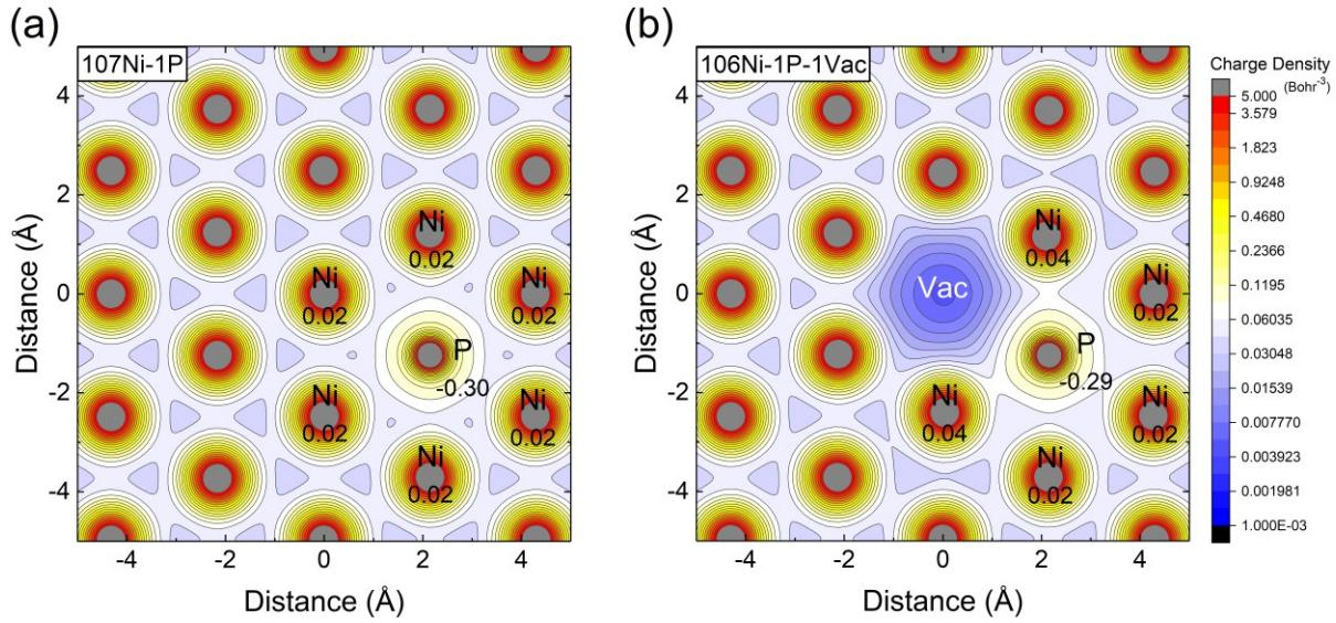
Figure 8. Contour maps showing the electron charge density (in a unit of Bohr<sup>-3</sup>) in the (111) plane
