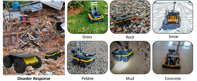
Figure 1. Motivating scenarios of robot adaptation to unstructured terrains. When mobile robots operate in a field environment during disaster response, the robots need the essential capability of navigating over a variety of terrains, such as grass, rock, snow, pebble, and mud, which often cannot be accurately structured before onsite robot deployment. In this paper, we propose the TRAL method to integrate representation learning and apprenticeship learning under a unified mathematical framework and estimate terrain feature importance to enable robust robot adaptation to unstructured terrains.
