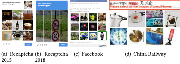
Figure 3: Examples of selection-based image captchas.
