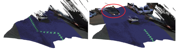
Figure 8 —Path Planning and Road Detection in Action: with extended vision, the oncoming vehicle and more road surface area is detected, and the path planner decides to not attempt overtaking.
