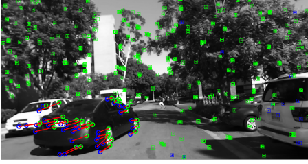
Figure 6 —Estimating the motion of a vehicle. The lines show the motion of features (represented by circles) across two successive frames.
