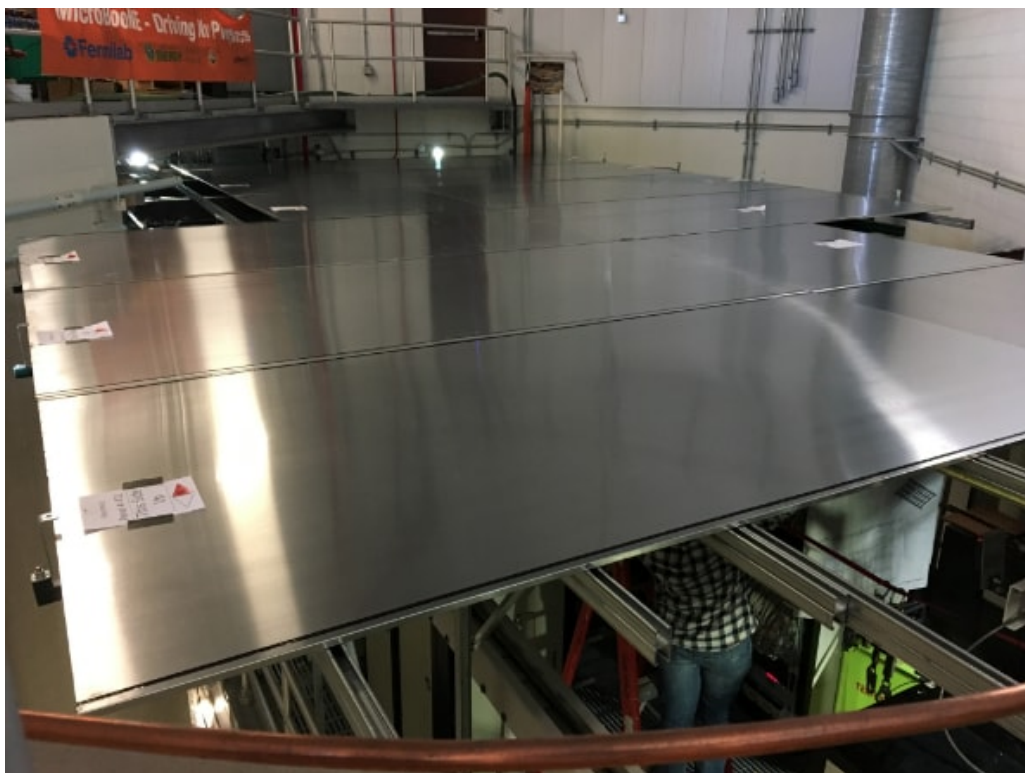
Figure 18. Completed MicroBooNE CRT top plane.
