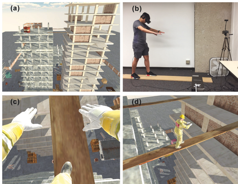
Fig. 4. Views in the virtual environment. (a) the perspective view of the overall virtual environment, (b) the real-world setup, (c) the first-person view in the virtual environment, and (d) a perspective view of the avatar.
