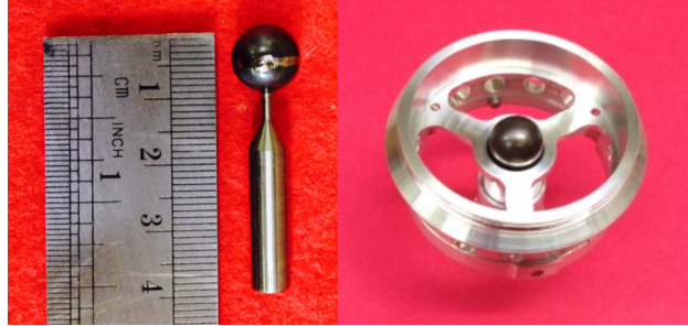
FIG. 6. Ti sphere used as container for the pressurized ^4\text{Ar} gas for irradiation (left), and the sphere target holder for irradiation at SARAF-LiLiT (right).
