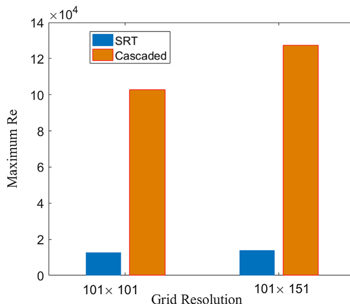
Fig. 15. Comparison of the maximum Reynolds number for numerical stability of single relaxation time (SRT) and cascaded LB methods for simulation of the shear driven swirling flow in a confined cylinder at different grid resolutions.
