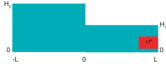
FIG. S5: Schematic illustration of the non-deformable cell considered here, consisting of two rectangles of unequal height. Active stress occurs in the right (front) rectangle.
