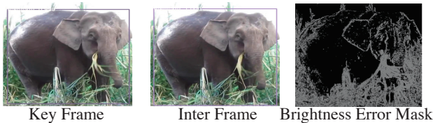
Figure 6: Brightness error computation mask.
