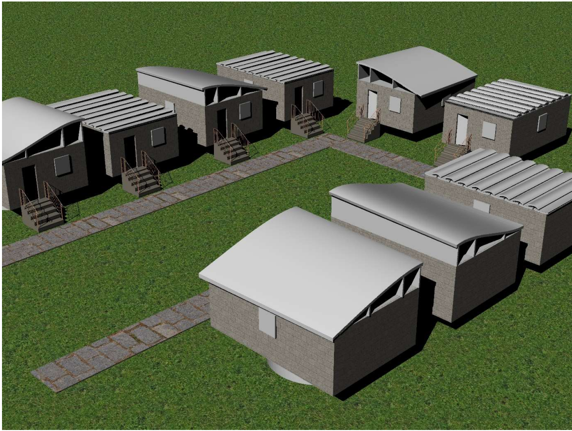
FIGURE 15. RETROFITTED AFFORDABLE HOUSING CONCEPT
