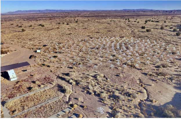
Figure 3. Aerial view of the LWA station at the Sevilleta National Wildlife Refuge. Most antenna elements are in a dense configuration towards the right of the image. A test antenna, is visible at the bottom. The signal processing hardware is contained within a modified, radio frequency shielded shipping container, visible in the left of the image.
