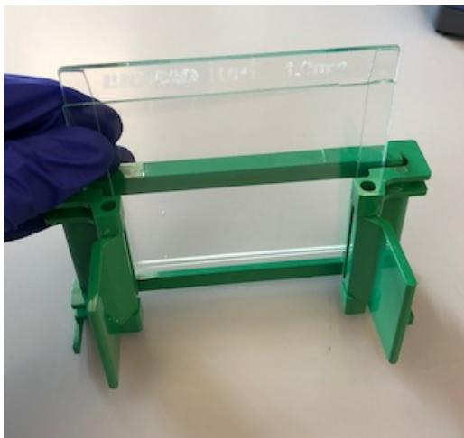
Place the entire assembly onto a Bio-Rad casting frame with the short plate forward and the casting frame seated with its base back touching the casting stand. Lock the plate/casting stand in place by engaging the spring-loaded lever on the top of the casting stand and applying pressure to the top of the spacer plate with the short plate oriented forward. Now it is ready for gel casting.
