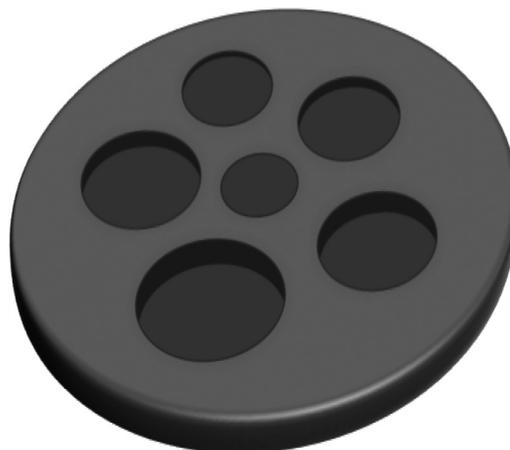
**FIG. 1.** Target design for the Ta baseplates used in this series. Each “pocket” cut in the baseplate creates a uniform step thickness. This allows six thicknesses to be studied per shot and improves uncertainties by correcting for reflections at the downrange surface. Reproduced with permission from Nguyen *et al.*, Phys. Rev. B **89** 174109,<sup>14</sup> Copyright 2014 American Physical Society.
