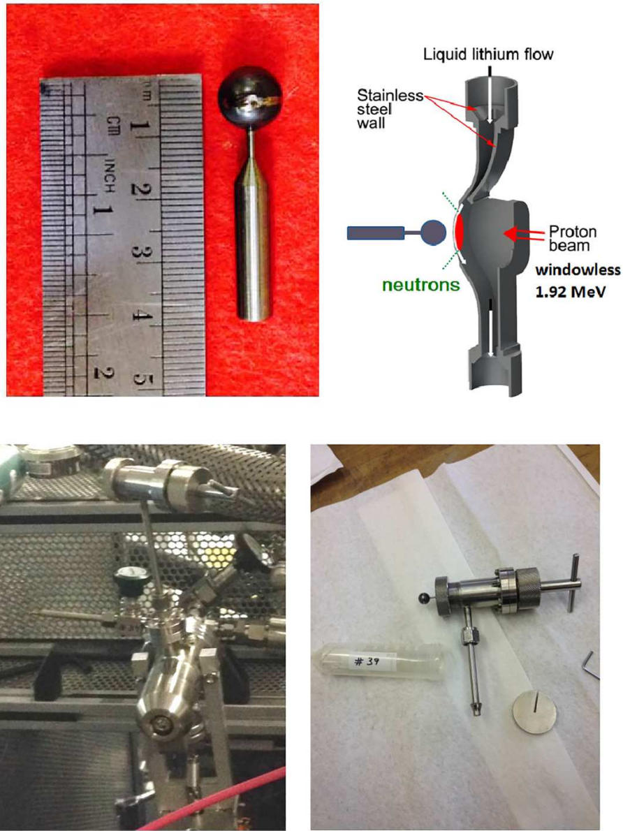
Fig. 6. (clockwise from top left) titanium sphere filled with isotopically enriched Ar ( \sim 25 bars); schematic diagram of the Liquid-Lithium Target (LiLiT): the proton beam ( \sim 3 kW) impinges (windowless) on a liquid-lithium film flowing in vacuum at a velocity of \sim 2.5 m/s to dissipate the beam power by transport. Neutrons with a quasi-Maxwellian energy distribution are produced at forward angles and irradiate the gas sphere; the gas-filled activated sphere mounted on a custom-made valve tool [18]; sphere and valve tool are installed on the ECR ion source port via a remote-controlled sapphire leak valve.
