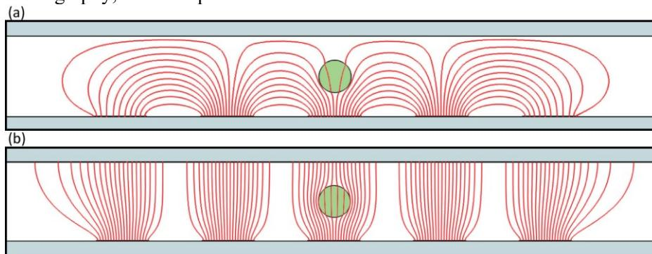
Figure 1: Simulation of the electrical field distribution generated by (a) coplanar-electrode sensor, (b) parallel-electrode sensor fabricated using our approach.
