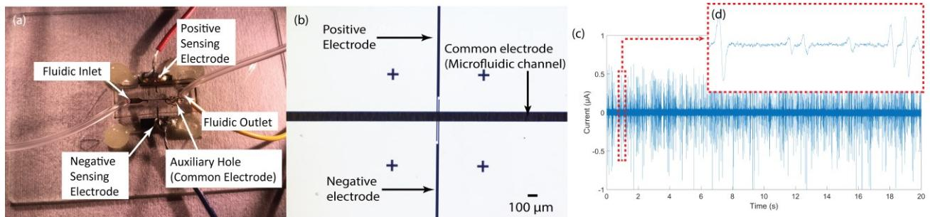
*Figure 3: Images of the fabricated microfluidic device and characterization results. (a) A photo of the fabricated device with fluidic and electrical connections and (b) a close-up of the parallel electrode sensor. (c) Approximately 2500 cancer cells were detected by the sensor during 20 s period. (d) A close-up figure showing the signals for 7 detected cells in 0.04 s.*
