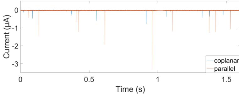
Figure 4: Resistive pulses recorded from a coplanar-electrode and a parallel-electrode sensor sequentially placed on the same microfluidic path with a  $15\text{ }\mu\text{m}$  channel height. The peak signal amplitudes generated due to the same cell are on average  $\sim 3.7\times$  higher for the parallel-electrode sensor. The result was found to be consistent with the finite element analysis results (not shown).
