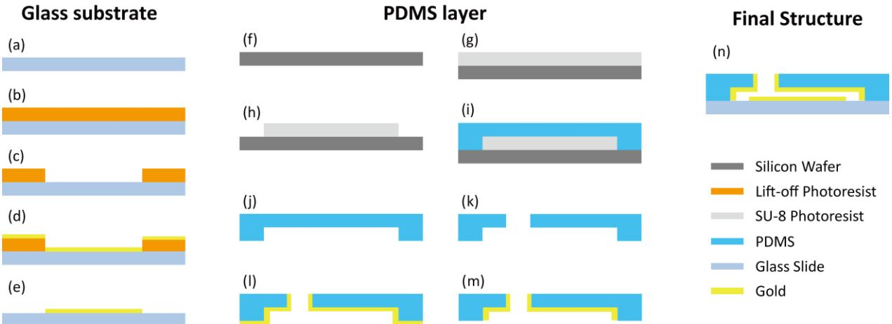
*Figure 2: The schematic showing the fabrication process to create parallel electrodes in a microfluidic device. (a)~(e) The fabrication of the glass substrate with micropatterned surface electrodes. (f)~(m) The fabrication of the metal-coated PDMS microchannel. (n) Bonding of the two components to form the final device.*
