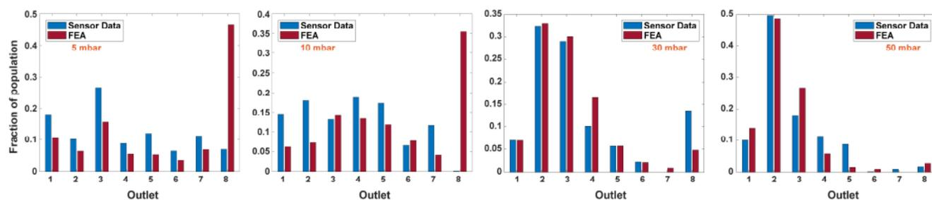
Figure 2: Comparison of experimental results obtained under different flow rates and finite element analysis results. Under low flow rates, some high expresser cells were trapped by the magnetic field. This led to an underestimation of the cell counts in the 8<sup>th</sup> outlet of 5 and 10 mbar experiments.
