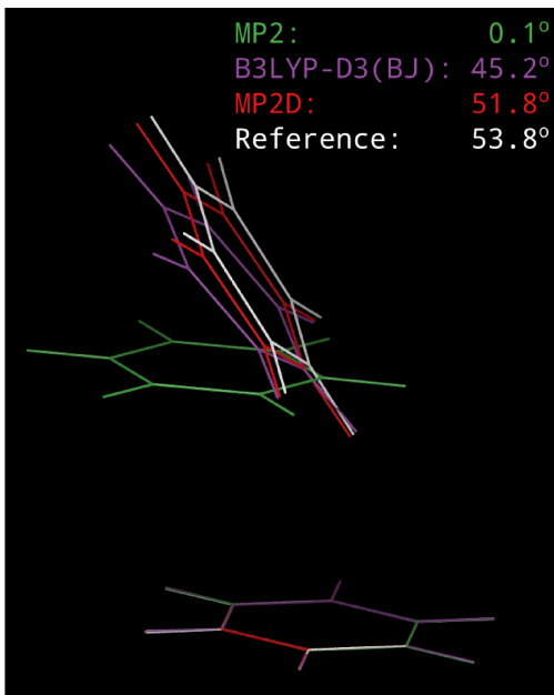
Figure 7: Overlay of benzene dimer S4, showing how MP2D (red) reproduces the correct angle between the molecules, unlike MP2 (green) and B3LYP-D3(BJ) (purple).
