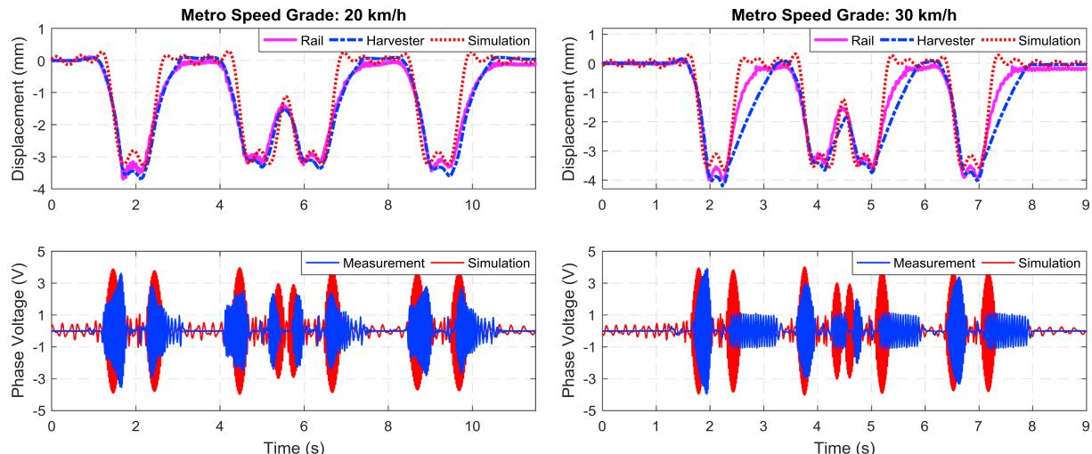
**Fig. 13.** Measured and simulated rail and harvester displacements and measured voltages at different vehicle speeds: (a) rapid transit train speed is 20 km/h and the external resistive load is 8 Ohm. The average power obtained in the test is 0.27 W; (b) rapid transit speed is 30 km/h and the external resistive load is 2 Ohm. An average 1.12 W was achieved in the test.
