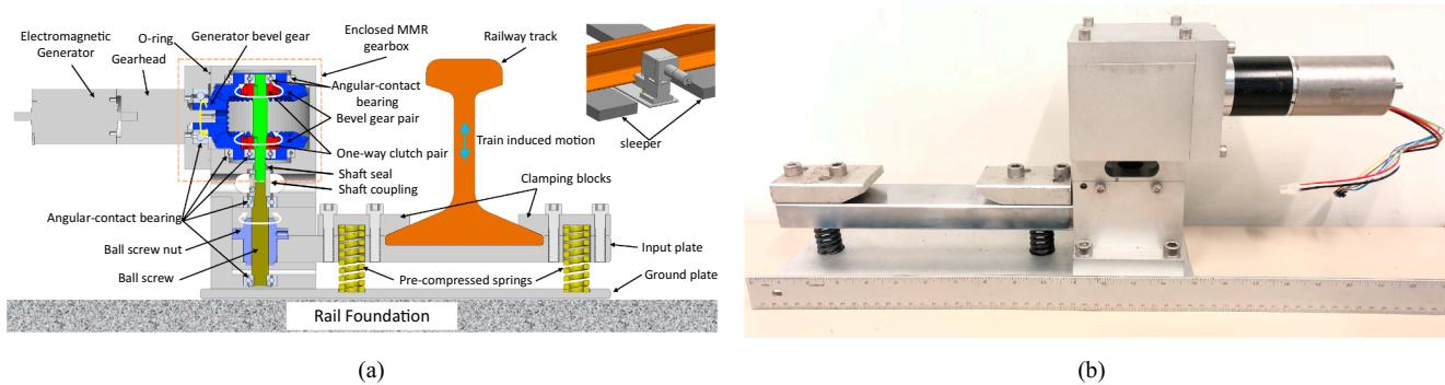
Fig. 1. Design of the ball screw based railway track energy harvester with MMR mechanism: (a) Design details (b) Prototype.
