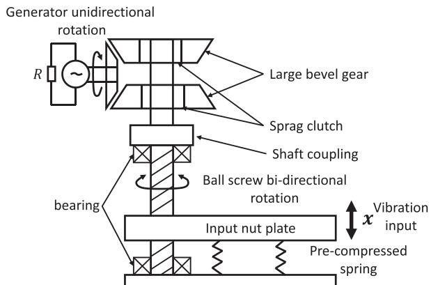
Fig. 4. Dynamic model of the proposed railway track energy harvester.
