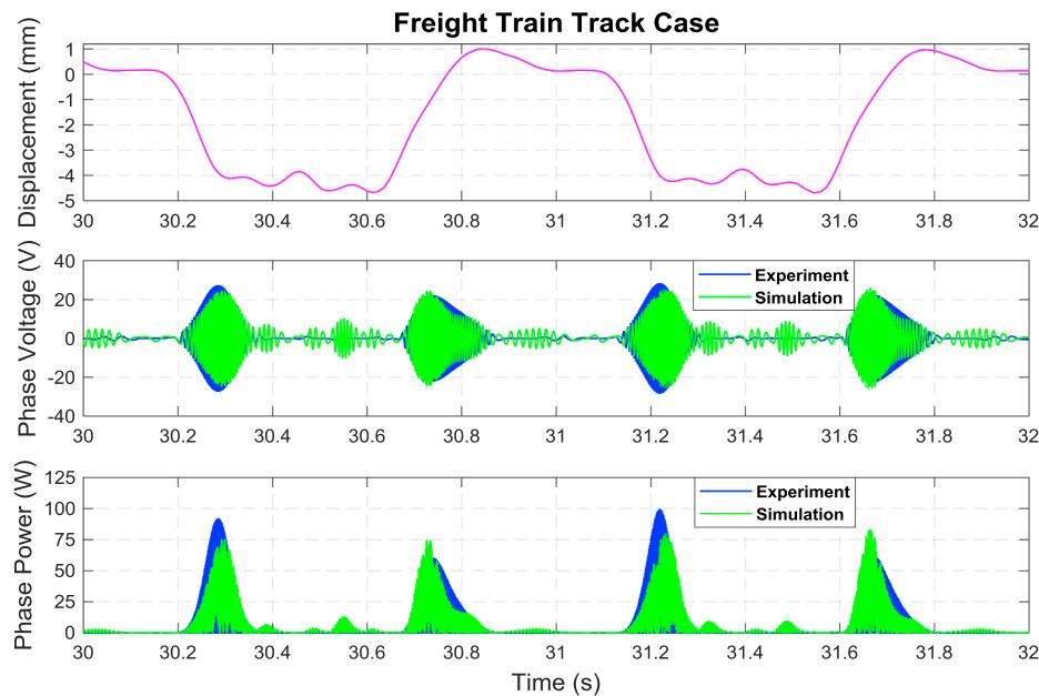
**Fig. 10.** Energy harvesting performance of the ball screw based harvester under measured freight train (running at 64 km/h) track displacement with 8 Ohm resistive loads in a Wye shape. The peak power in a single phase is 114.98 W and the average power in all three phases are 17.50 W.
