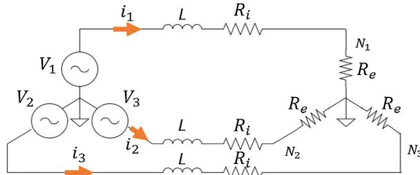
Fig. 3. Modeling of star shape three-phase generator with star shape resistive load [29].
