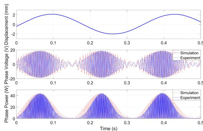
**Fig. 9.** Measured and simulated phase voltage and power of harvester prototype 2 under sinusoidal excitation with amplitude  $\pm 2$  mm and frequency 3 Hz. The harvester is connected with an 8 Ohm resistive loads in Wye shape and the average power of the total three phases is 26.61 W.
