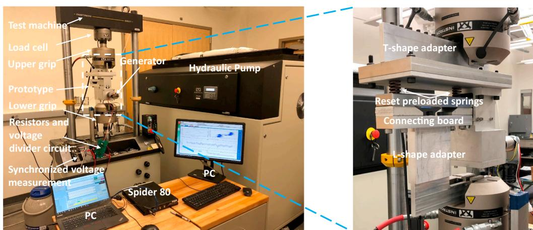
Fig. 8. In-lab experiment setup.
