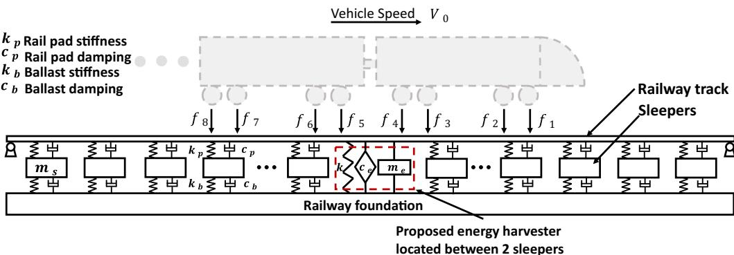
Fig. 5. Dynamic model of Train-track-harvester system.
