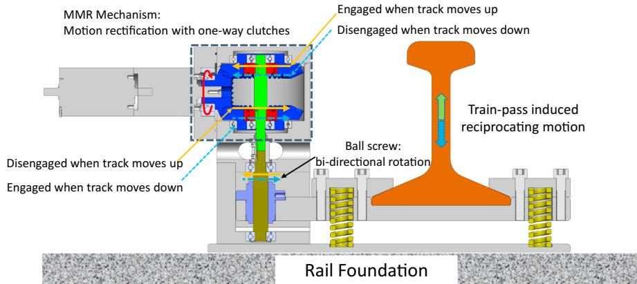
Fig. 2. Bidirectional vertical track motion induced by wheel-rail vertical contact force will drive the generator to rotate in one direction using the proposed ball screw MMR mechanism: green lines represent the case that track moves up and blue lines represent the case that the track moves down.
