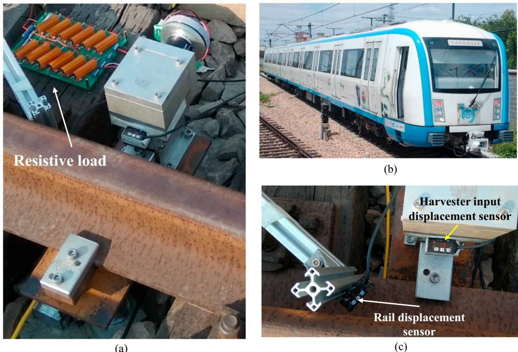
**Fig. 12.** In field test setup: (a) Harvester prototype 1 was clamped on the railway track and positioned between two adjacent sleepers. (b) A two-unit Type A rapid transit ran with a speed of 20–30 km/h; (c) Two laser displacement sensors measured the railway track displacement and harvester input displacement, respectively.
