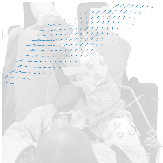
Fig. 4. Image showing the modeled direction of force produced at the wrist by the deltoids throughout the workspace. The direction of force changes based on the position and orientation of the wrist.
