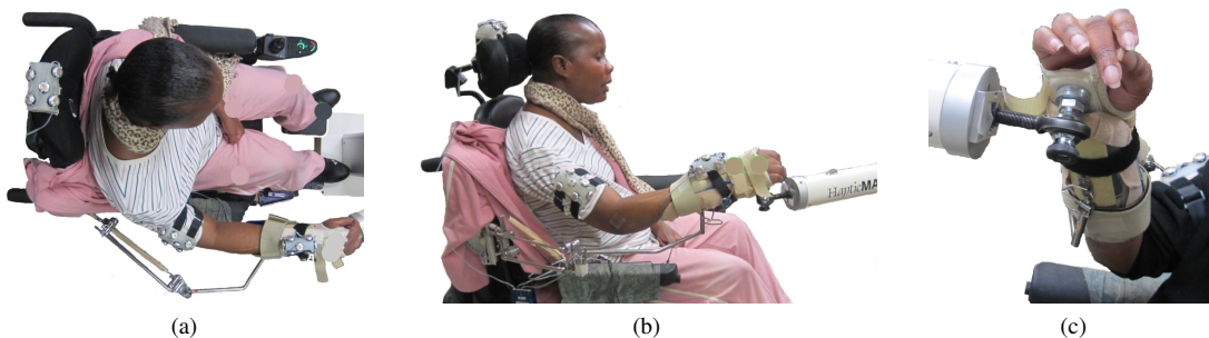
Fig. 1. Instrumentation for experiments. Pictured is the participant's right arm. Shown in (a) and (b) are the placement of reflective markers for optical tracking, a passive arm support providing supporting force, and the robot that drives the participant's wrist to 27 positions in the participant's workspace. The participant's wrist and distal forearm (c) are in a soft cast that is attached via a magnet to a ball-and-socket joint at the end effector of the HapticMaster robot.
