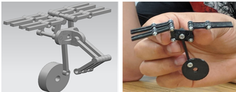
Figure 3. Hybrid actuation mechanism FWMAV 1.
