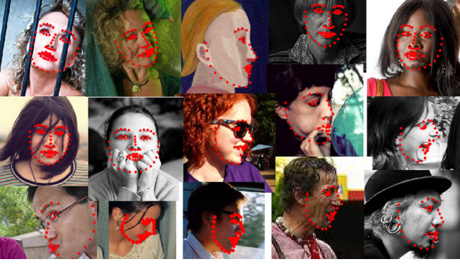
Fig. 3: Example landmark detection from OpenFace 2.0, note the ability to deal with profile faces and occlusion.
