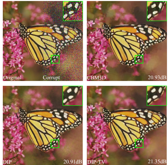
Fig. 1: Comparison of DIP-TV against several standard algorithms for image denoising. DIP-TV achieves the best SNR performances on Monarch with AWGN of \sigma = 65 . The combination of the CNN and TV priors preserve homogeneity of the background as well as the texture, highlighted by rectangles drawn inside the images.
