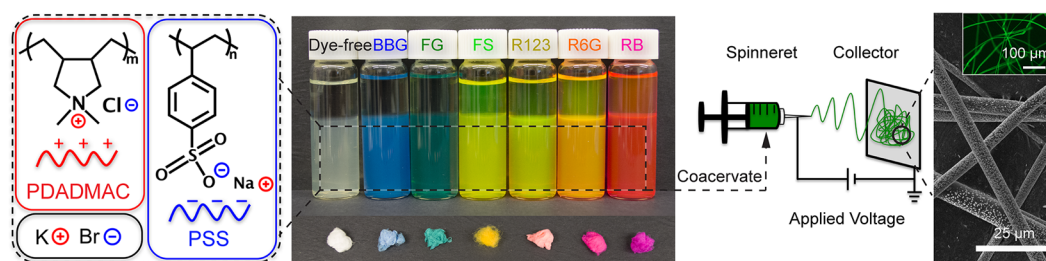
Figure 2. Schematic of the process used to electrospin the coacervate phase into polyelectrolyte complex (PEC) fiber mats. Dye-free complex coacervates composed of poly(4-styrenesulfonic acid, sodium salt) (PSS), poly(diallyldimethylammonium chloride) (PDADMAC), and potassium bromide (KBr) in water and coacervates containing brilliant blue G (BBG), fast green FCF (FG), fluorescein sodium salt (FS), rhodamine 123 (R123), rhodamine 6G (R6G), and rhodamine B (RB) were electrospun. The polymer-rich coacervate phase was used as the electrospinning precursor solution. The SEM and fluorescence micrographs show FS-containing PEC fibers.
