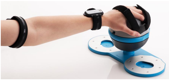
Fig. 1. The Bimeo arm rehabilitation system, which consists of two inertial sensors on the arm as well as an inertial sensor inside a handheld module.
