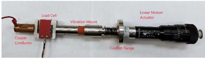
Fig. 9. Contact bolted to linear motion actuator
