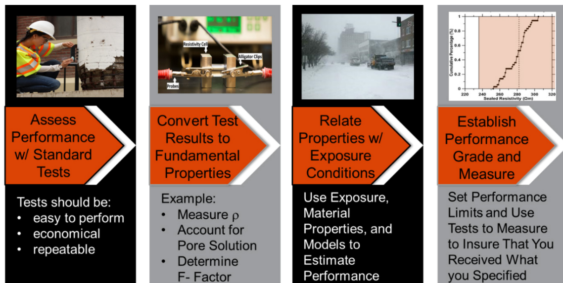
Figure 1: Four-stage approach to relate simple standard test methods to fundamental properties and utilize these properties with exposure conditions to perform simulations that enable performance grades to be established and compared with field quality acceptance measurements [24].
