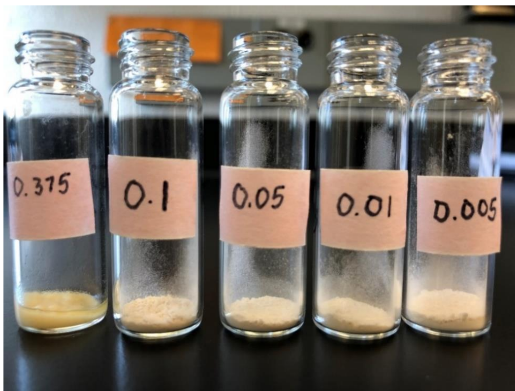
Figure S1. Bulk morphology of M-MFI(P) after TEOS intercalation in the VPP process. The mass ratio of TEOS/M-MFI(P) was controlled to (1) 3.75, (2) 1.00, (3) 0.50, (4) 0.10 and (5) 0.05, respectively. The numbers in the label of each glass vial is TEOS mass (unit: gram). (synthesis conditions: 343 K, M-MFI(P) = 0.1 g and mass ratio of H 2 O/M-MFI(P) = 10 in the hydrolysis step)
