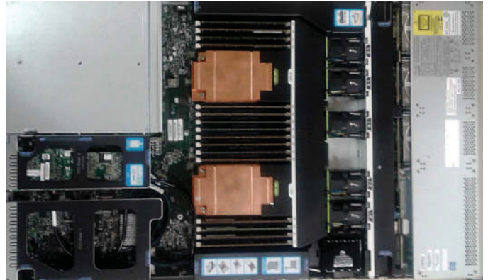
Figure 2: Cisco UCS C220 M3 server (air-cooled)
