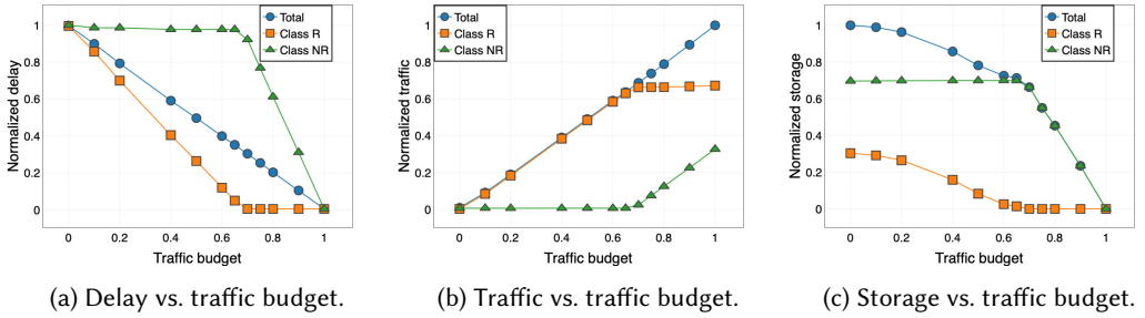
Fig. 12. Minimize delay with a constraint on traffic. Keys with higher unit delay cost ( d_k^m ) are always given preference over the keys with lower unit delay cost in the assignment of available traffic budget.
