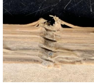
c) screw type D following removal of screw
