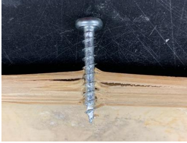
a) screw type D ( t = 6.9 mm)
