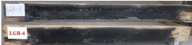
b) after fire tests (top:LGB-3; bottom: LGB-4)
