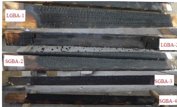
b) specimens following fire conditioning
