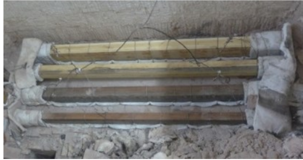
a) specimens in furnace before fire exposure
