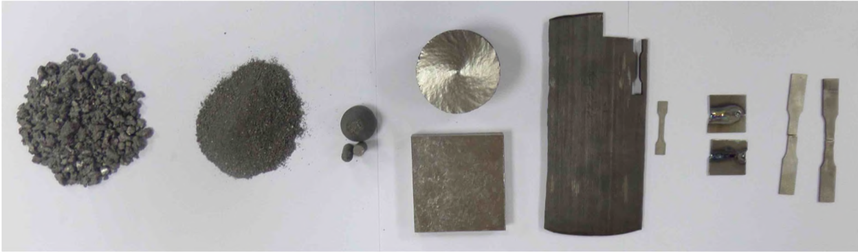
Fig. 12. Samples of ULR titanium at the different stages of production, from left to right: 1. ULR titanium sponge; 2. magnetically separated crushed sponge; 3. isostatic compacted sponge; 4. vacuum arc-welded (cylinder) and electron-beam melted (rectangular block) ingots; and 5. samples for mechanical tests.
