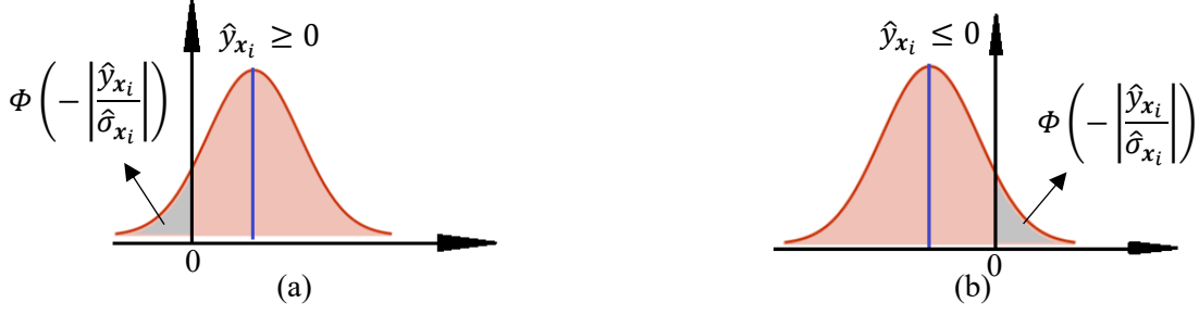
Fig. 1. An illustration of the probability of wrong sign estimation in Eq.(18) considering (a) \hat{y}_{x_i} \geq 0 or (b) \hat{y}_{x_i} \leq 0 .
