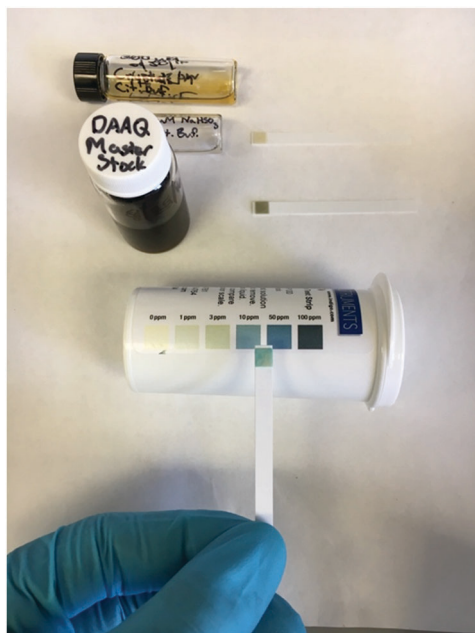
Fig. 5 Test strip dipped into the reoxidized 300 \mu\text{M} DAAQH 2 solution in the top vial, showing the presence of hydrogen peroxide in the expected amount (300 \mu\text{M} , i.e. 10.2 ppm). The middle vial contains a 300 \mu\text{M} solution of sodium bisulfite and the bottom vial contains a 1.2 mM solution of DAAQ that had not been subjected to the redox reaction.
