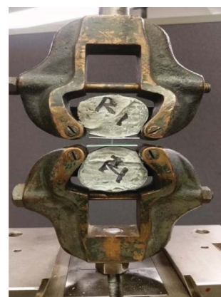
(b) Bond test setup
