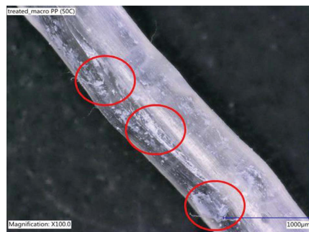
(c) Dried at 50°C after sol-gel treatment(OMP)
