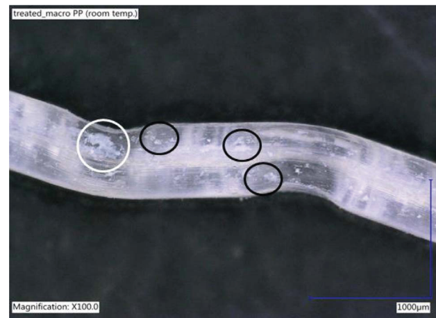
(b) Dried at room temperature after sol-gel treatment(RMP)
