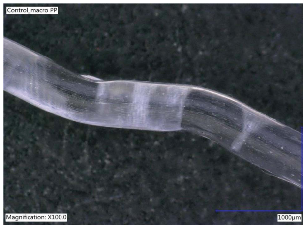
(a) Untreated structural polymer fibre (UMP)
