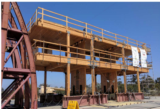
Fig. 1. Full-scale wood building with coupled rocking CLT walls designed by Kattera. (Image by S. Pei.)
