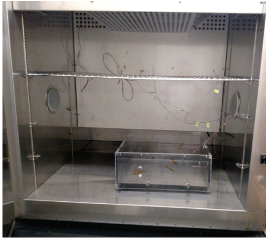
Fig. 18 Accelerated thermal cycling trial testing setup in environmental chamber
