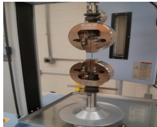
Fig. 15 Test setup to measure mechanical properties of cable specimen
