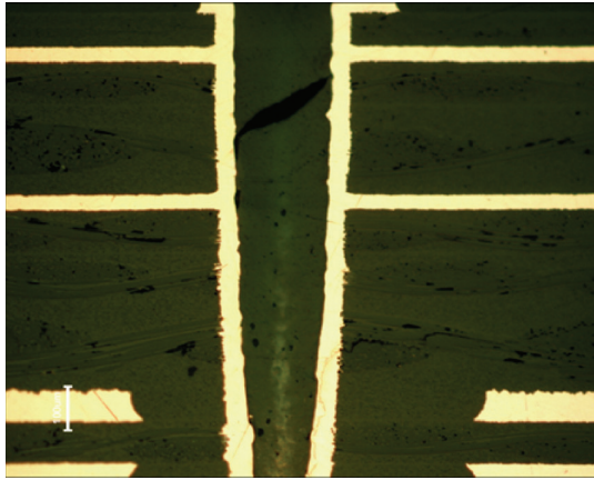
Fig. 5 Cross section of PCB plated through-hole on oil exposed server
