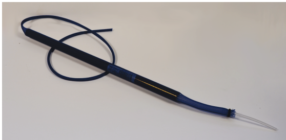
Fig. 3. The jig used to sheath the bladders with the expandable sleeving. Without the jig, the sheathing constricts around the compliant actuator and sticks before reaching the end. The molded bladder fits inside the tube, while the sheath fits over the outside, and both are pulled away together.
