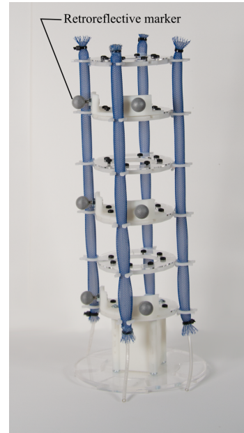
Fig. 5. A single-segment arm ready for testing. The lowest radial support plate was bolted to a rigid base, to set a consistent boundary condition. Retroreflective markers were attached to the radial support plate via bracket adapters printed on a FormLabs, replacing the acrylic top plates.
