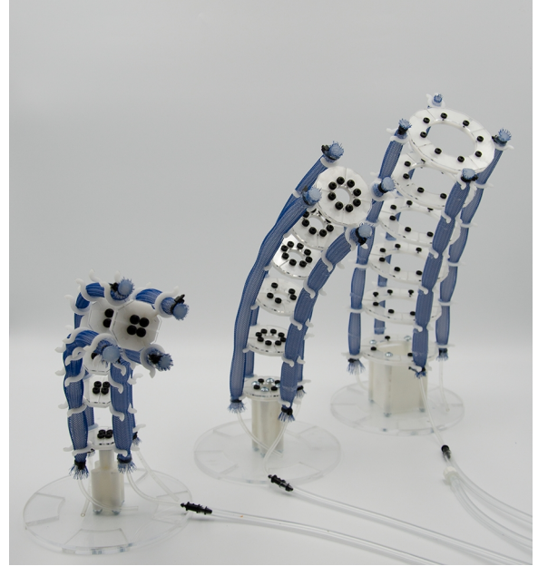
Fig. 1. Three segments developed for testing, pressurized to their (approximately) minimum bend radius. The design of each of the McKibben actuators is the same, but the diameter of the arm varies. From left to right, the arm diameters are: 45 mm, 60 mm and 90 mm.
