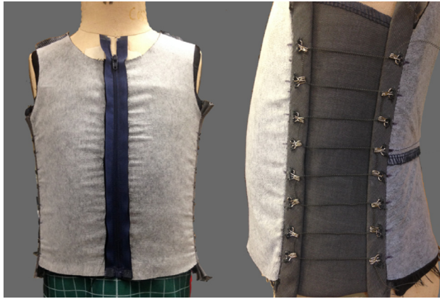
Fig. 2 Photograph of the SMA-actuated compression garment front (left) and side view (right)
