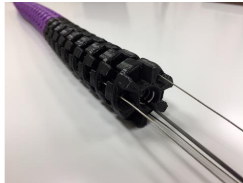
Figure 11. Construction of the support branches ("elbows")
