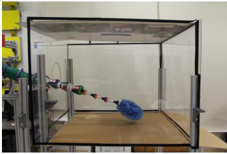
Figure 15. Mock-up glove box with robot entering through port on left
