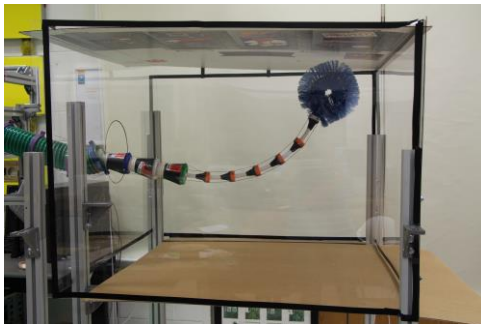
Figure 16. Robot reaching to clean top and corner of box
