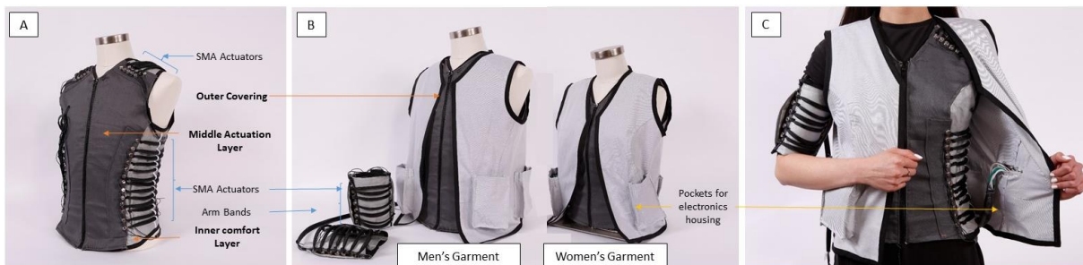
Figure 1. Garment-based dynamic compression system components and design. (A) Inner comfort layer and middle actuation layers; (B) Final men's and women's garment design with arm bands; (C) Women's garment worn on the body showing all system components
