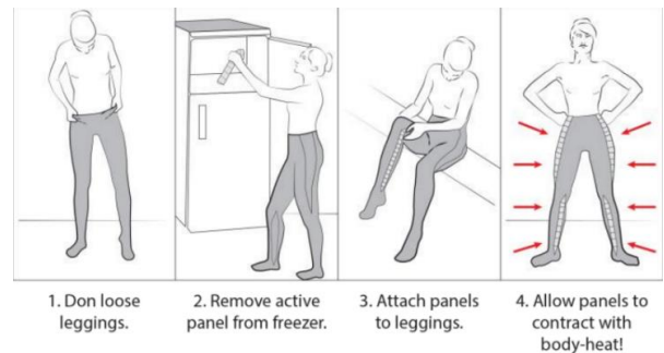
FIGURE 2: LOW-TEMPERATURE-ACTUATED SMA COMPRESSION GARMENT THAT ACTIVATES AT ROOM/BODY (ORIGINALLY APPEARED IN GRANBERRY ET AL) [10].
